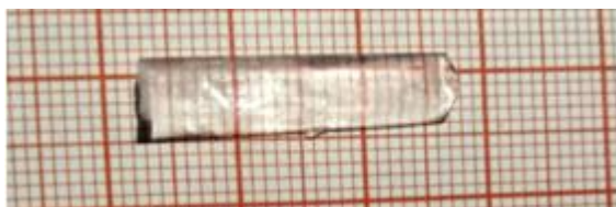
Fig.2 The grown bulk single crystal of LPT
